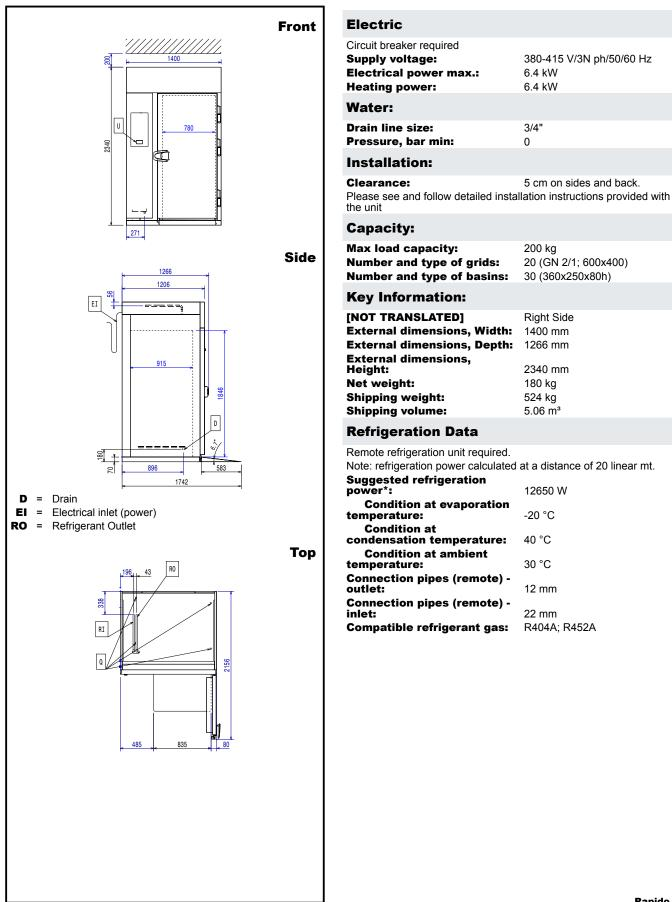
Rapido Blast Chiller-Freezer 20GN2/1 200/170 kg with Floor Ra The company reserves the right to make modifications to the products without prior notice. All information correct at time of printing.
